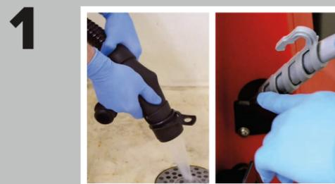
Drain the solution tank of contents and rinse with water until drainage is clear.
