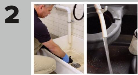
Drain the recovery tank into an approved drain location. Rinse the tank thoroughly to remove all dirt and debris.
