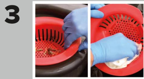
Clean and disinfect the inside of the recovery tank and debris tray.
