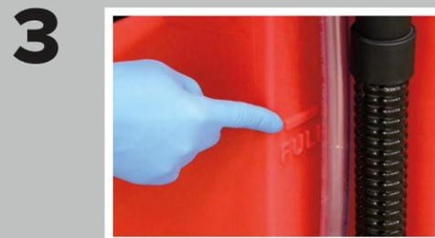
Fill the solution tank to max capacity and let dwell per the labels instructions.
