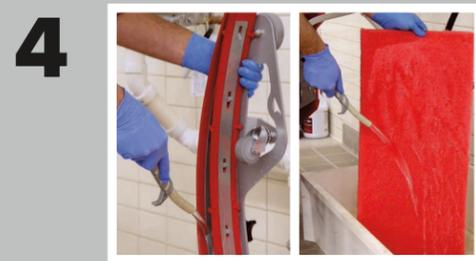
Remove the squeegee, pad drivers or brushes and rinse off each thoroughly – ensuring there is no visible debris. Spray each with Betco® disinfecting cleaners and allow proper dwell time.
